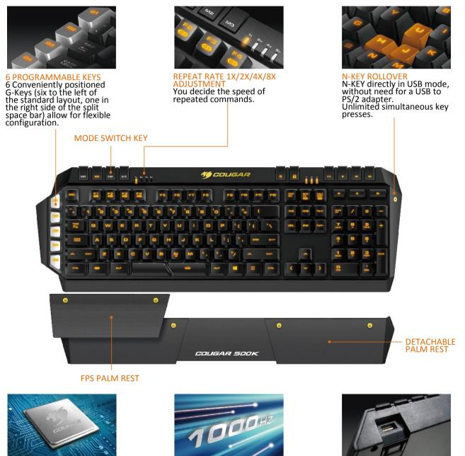
32-BIT ARM PROCESSOR Superior computing speed, instant response and smooth operation. ON-BOARD MEMORY Store up to 3 full configuration profiles on the keyboard and bring your settings anywhere you want.
